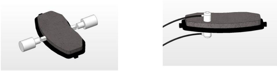
Figure 2a) In-plane coupling configuration; b) through-the-thickness configuration.
